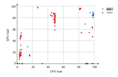
Figure 1. Comparison of average CPU and GPU load (in percent) for the jobs of the selected user and all other users of GROMACS package. Each dot represents one job
